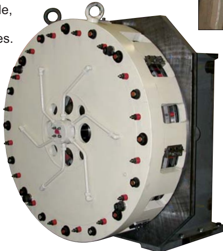
Dry Friction Clutch on Test Stand
