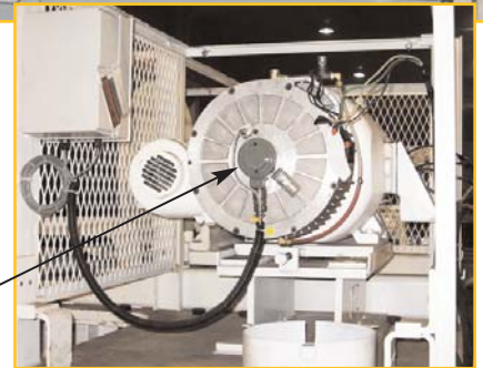
External Encoder Mounting For Easy Access
