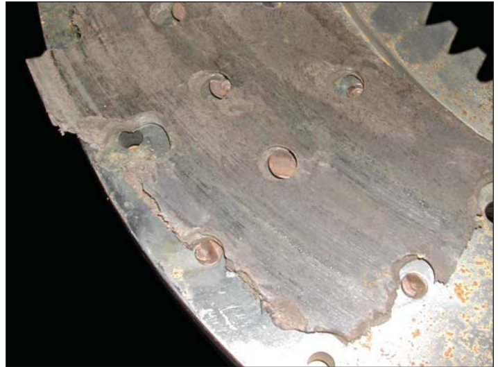
Damaged Riveted Plate
