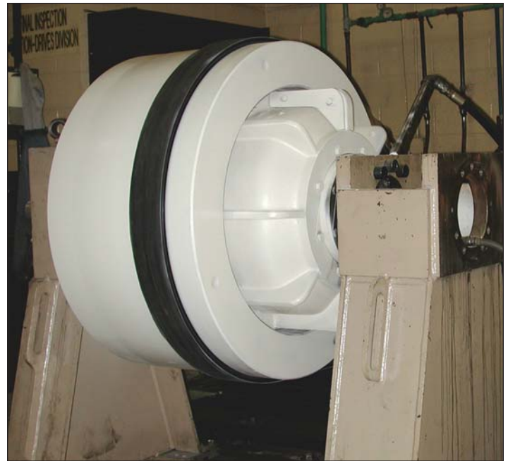
Press Pac® 2161 Series - Integral Unit on Test Stand
