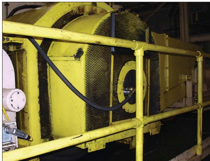
Press Pac® 3294 Series – Hydraulic Actuation / Oil Cooled
