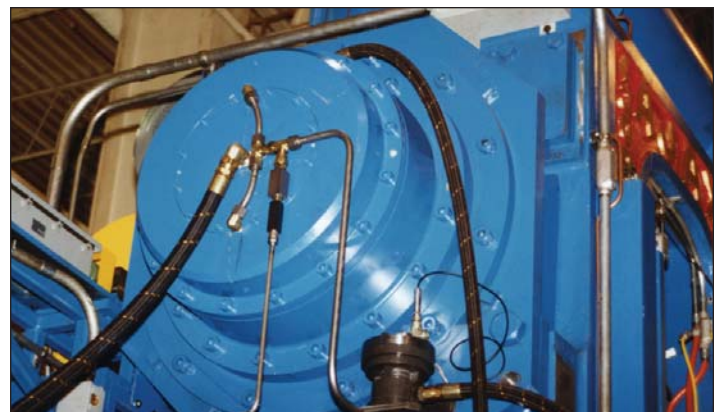
Press Pac® Brake Only Application Ajax® 1300 Ton Forging Press Application
