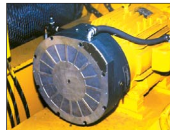
Step 4 – Wire Brake to Motor
