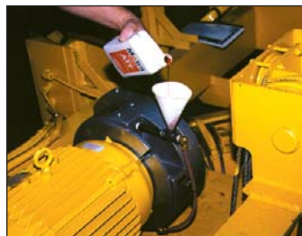
Step 3 – Fill Brake Using Type F Fluid
