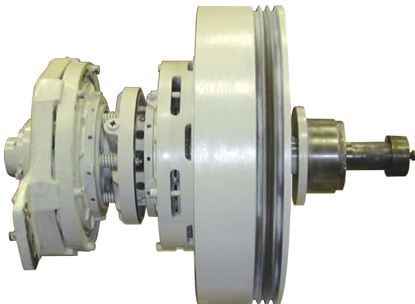
Verson* Clutch/Brake Repaired and Ready for Shipping
