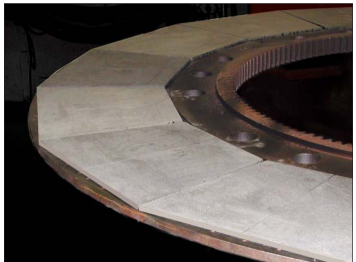
114" Clutch Plate Bonded With Thermal Adhesive Bonding Technology
