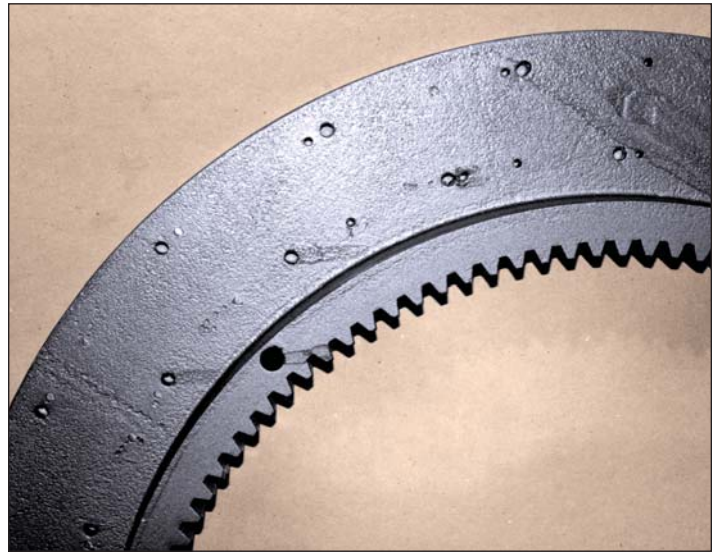
Riveted Plate in For Reline – Weakened Structural Integrity
