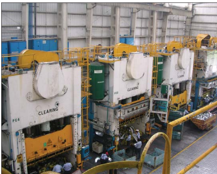
Tier 1 Automotive Stamping Plant Retrofitted With Press Pac® Hydraulic Clutch/Brakes
