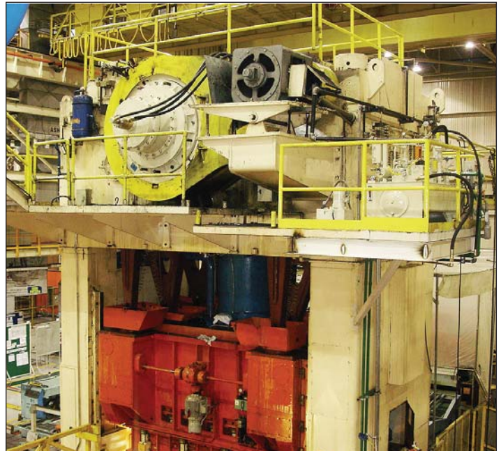
Press Pac® 2297 Separate Clutch & Brake Danly® 1600 Ton Double Action Stamping Press Installation
