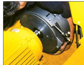
Step 2 – Slide Brake on Motor Shaft
